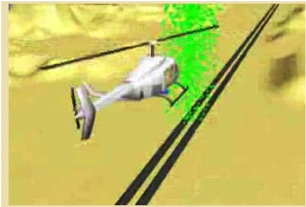
Figure 4. Simulation of ATS’s helicopter over a pipeline with the methane plume indicated in green.
